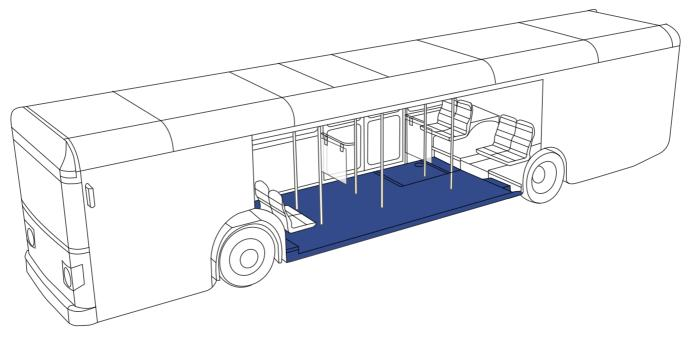
3A Composites Mobility produces **extremely light and stiff composite chassis floors with integrated functions**. The chassis floors can also be made significantly thinner than the conventional floors due to the high stiffness.
