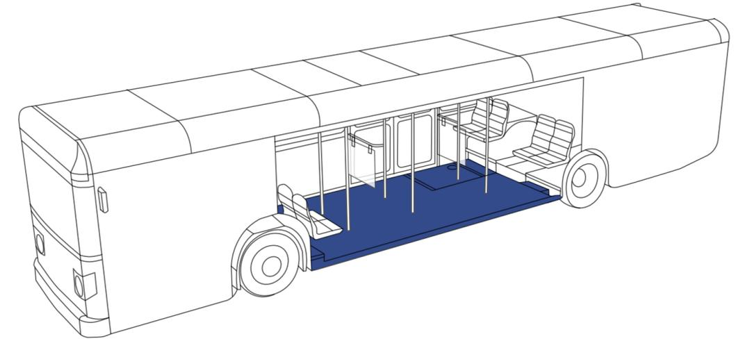
3A Composites Mobility produces **extremely light and stiff composite chassis floors with integrated functions.** The chassis floors can also be made significantly thinner than the conventional floors due to the high stiffness.
